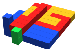
■ Figure 62 Cooperative binding for direction ‘1’ tile growth of the first tile in row 2 extends to the edge of the base. A direction ‘1’ detection gadget (green) attaches to the base and the growing row, indicating the edge has been reached. Once the direction ‘1’ detection gadget is bound, a glue activates on the +y face of the tile, allowing for cooperative growth in the +y direction on the currently grown structure.
